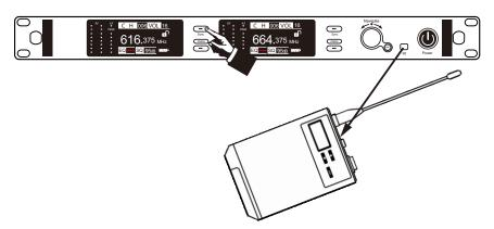
Align the infrared frequency matching window of the transmitter with the infrared frequency matching window of the receiver(within 20cm distance), press the frequency matching button of the receiver, after the frequency matching is successful, the display screen of the transmitter will shine and the frequency will become consistent with the receiver, that is, the frequency matching is successful.
