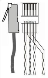
Notice: Cable connectors MUST be metal one, the shielded layer of cable MUST be connected to the connector's metal shell, to make a better
