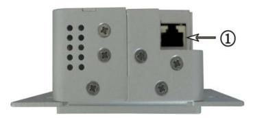
① HDBT OUT: RJ45 port, connect with receiver via a CAT5e/6 cable to deliver Audio/ Video signals, support PoC.
